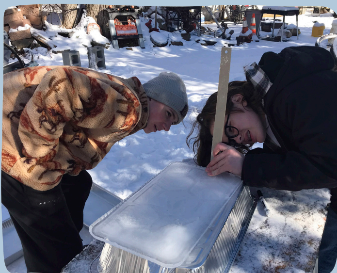
Jack and Lee discovered that their ice froze quite unevenly in the farmhouse freezer. They compensated for this potentially confounding variable by carefully measuring their ice blocks on each corner and averaging the thicknesses.
