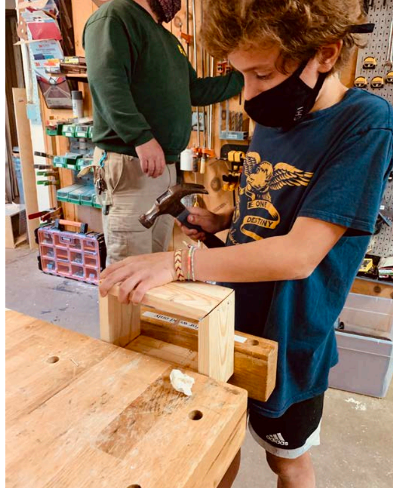
Silas taps in small brads to attach the corners of the wooden picture box he built during Tuesday Group II.
