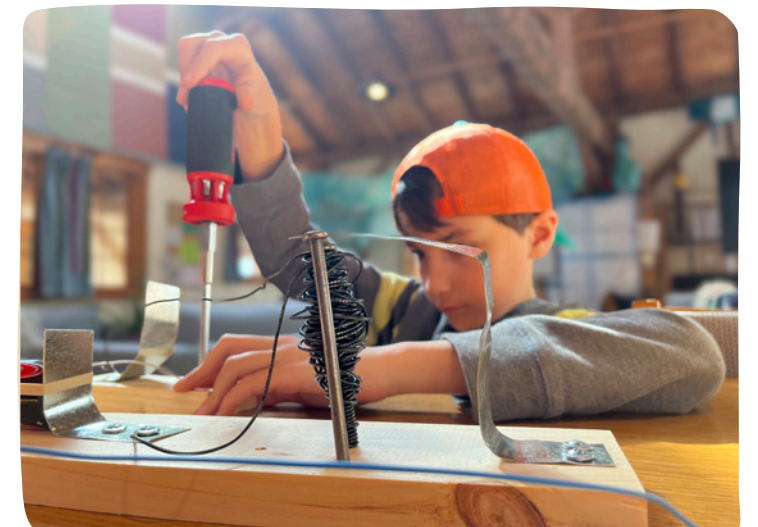
Marlon tightens the connections on the key for the telegraph he is constructing as part of Choice A: Industrial Revolution. As part of this project, youth also explored some of the history of communications technology, Morse code, basic circuitry, and electromagnets.
